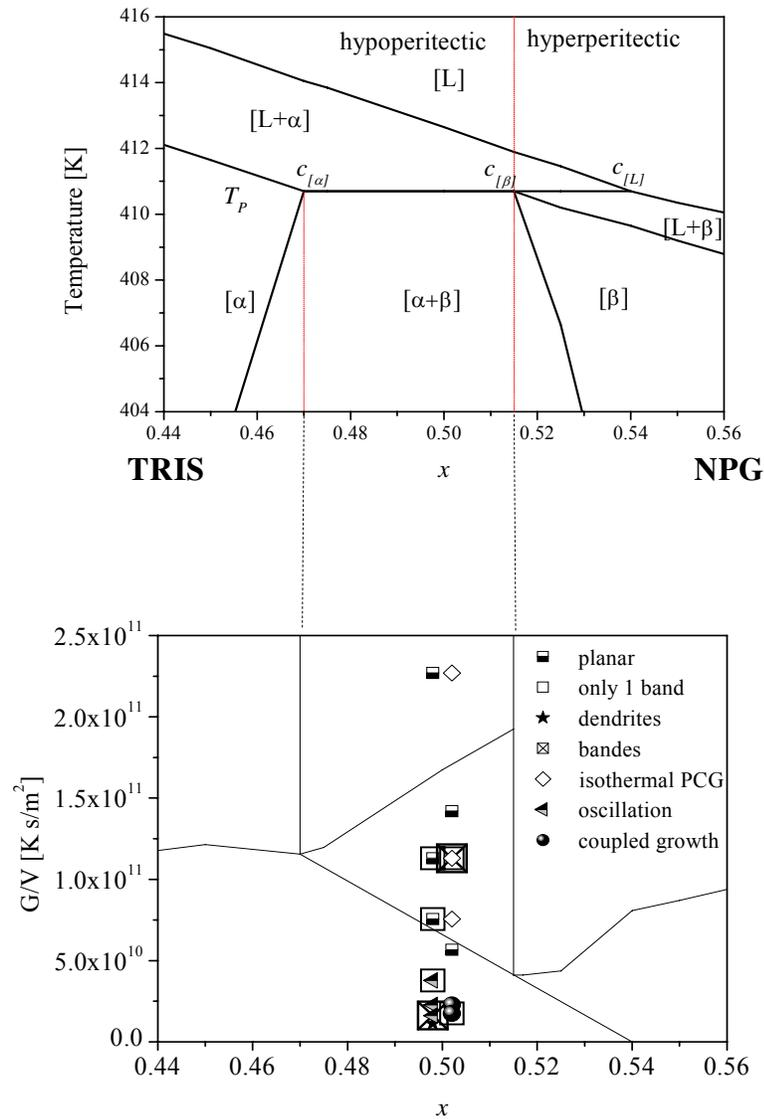
Figure 5: Peritectic region of the phase diagram and calculated microstructures depending on the applied  $G/V$  and the mol fraction  $x$  as full lines. The solidification morphologies for a hypoperitectic concentration are given as symbols. Experiments with a initial planar front are in the left column and results with a dendritic/cellular initial interface are on the right one.
