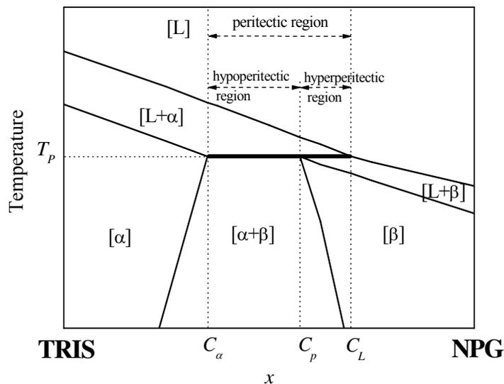
Figure 1. Detail of the TRIS –NPG phase diagram. At the peritectic temperature  $T_p$  and the peritectic concentration  $C_p$  the primary  $[\alpha]$  phase, the peritectic  $[\beta]$  phase, and the liquid phase  $[L]$  are in equilibrium.
