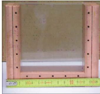
**Figure 1.** Rectangular cavity used for controlled solidification experiments. The inner dimensions are  $10 \times 10 \times 1 \text{ cm}^3$ .
