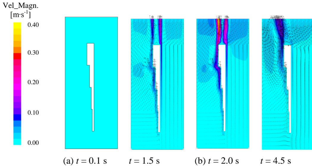
**Figure 4:** Contour of velocity magnitude and velocity vectors of the liquid phase in the (a) film boiling regime ( $t \leq 1.53$  s) and (b) the nucleate boiling regime ( $t > 1.53$  s)
