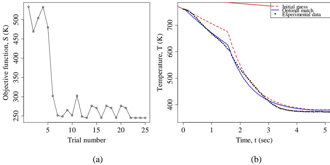
**Figure 2:** Evolution of the objective function  $S$  (a) and the cooling curves for the initial guess and final solution compared to experimental data at thermo couple 2 (b)
