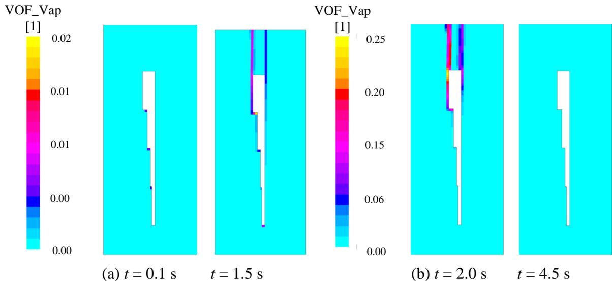
**Figure 3:** Phase fraction of the vapor phase in the (a) film boiling regime ( $t \leq 1.53\text{ s}$ ) and (b) during the nucleate boiling regime ( $t > 1.53\text{ s}$ )
