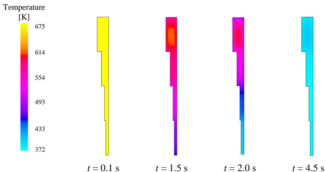
**Figure 5:** Contour of the casting temperature at different moments, the initial temperature of the casting is 761.19 K.
