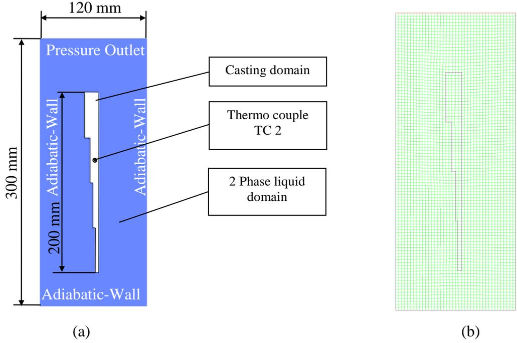
**Figure 1:** (a) Computational domain and boundaries with the position of the thermocouple 2 within the 10 mm step and (b) corresponding structured grid.
