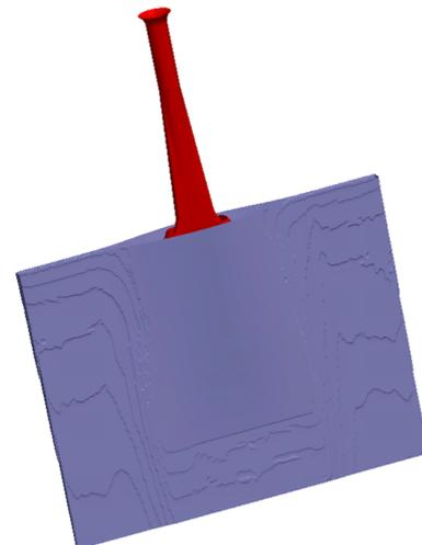
Figure 17: Formation of the solid shell in the TS caster simulated with the improved model
