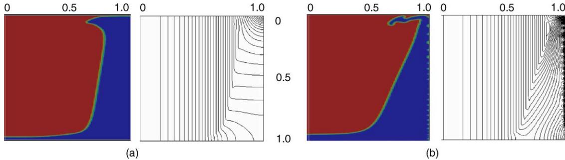
Fig. 7. The phase and electric current distributions just at the moment when the interface reaches the electrode leading to an electrical shortcut,  $k = +\infty$  (a) and  $k = 0.1$  (b) ( $R_2/R_1 = 1$  and  $H/R_1 = 1$ ).
