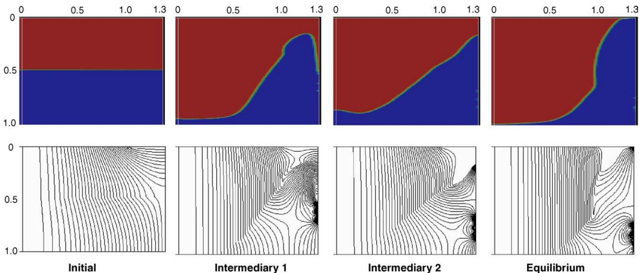
Fig. 5. Evolution of the phase (upper) and the electric current (bottom) distributions in the  $r$ - $z$  plane for a conducting mould with  $k=0.1$ ,  $R_2/R_1 = 1.3$  and  $H/R_1 = 1$ .
