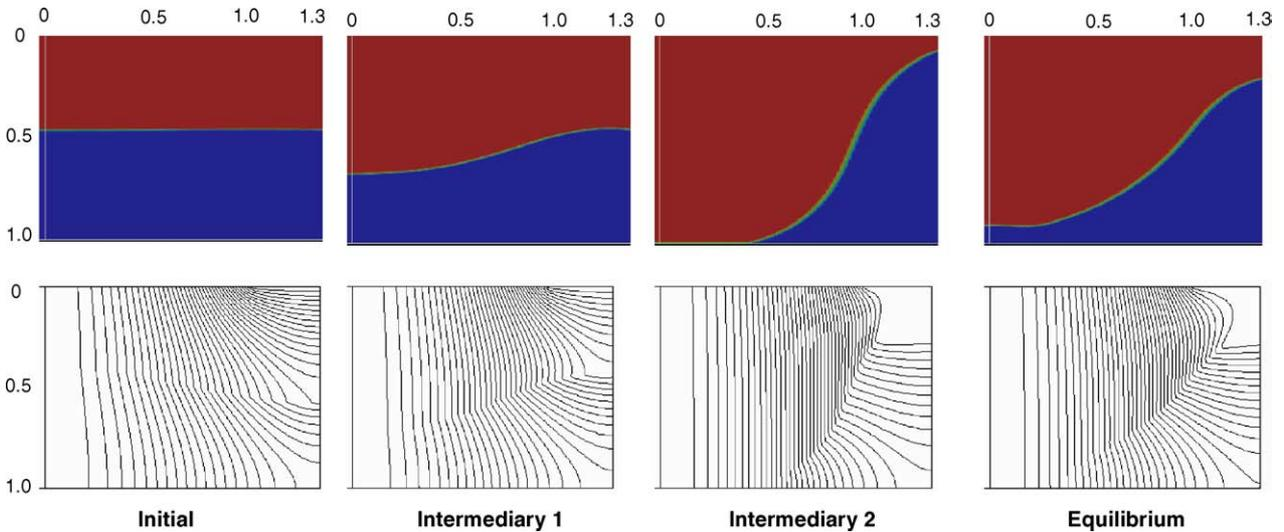
Fig. 4. Evolution of the phase (upper) and the electric current (bottom) distributions in the  $r$ - $z$  plane for a perfectly conducting mould ( $k=+\infty$ ) with  $R_2/R_1 = 1.3$  and  $H/R_1 = 1$ .
