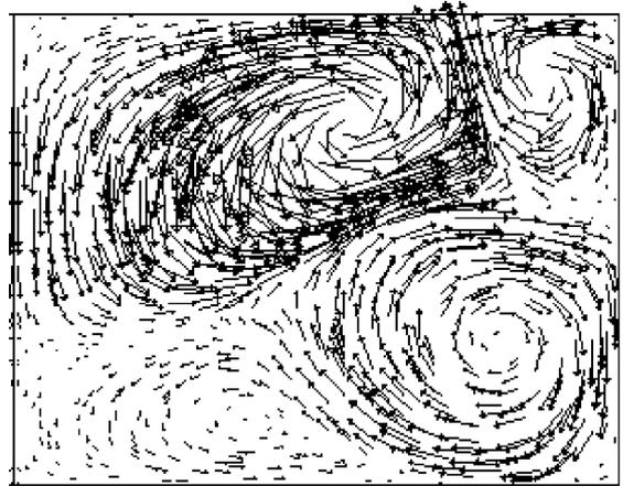
Fig. 2. The velocity field at the equilibrium state in the  $r$ - $z$  plane for  $k=0$  and  $R_2/R_1 = 1.3$ .
