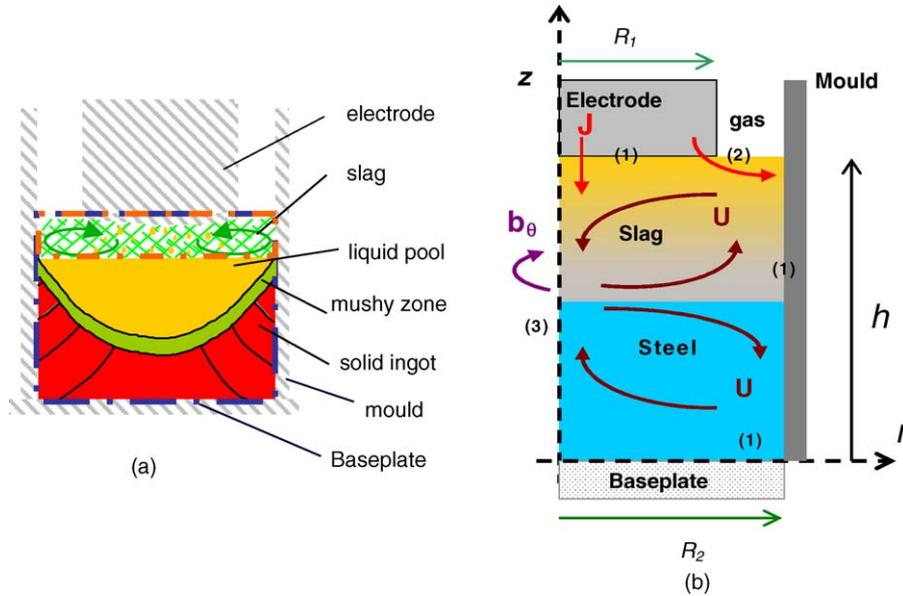
Fig. 1. (a) Schematic representation of an ESR system. (b) Geometry of calculation domain and flow boundary conditions. At the walls:  $\vec{u} = 0$  (1). At the slag/gas interface:  $\partial \vec{u} / \partial z = 0$  (2). At the axis of symmetry  $u_r = 0$  and  $(\partial u_z / \partial r) = 0$  (3).
