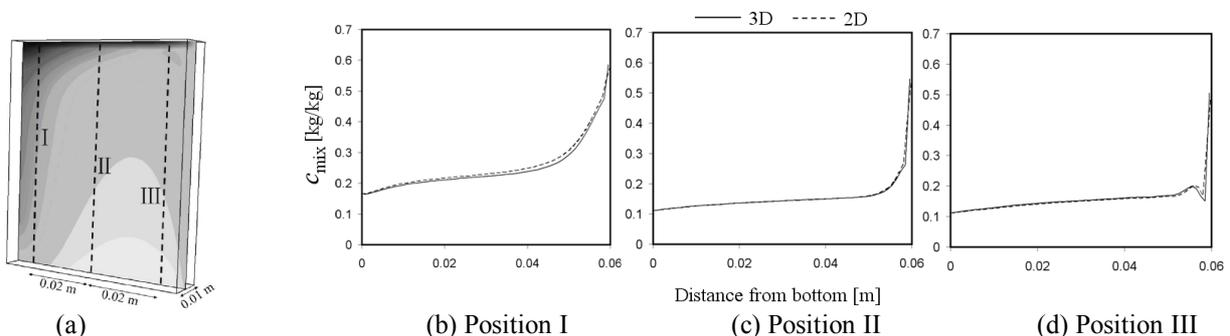
Fig. 2 Comparison of 2D and 3D calculations. (a): Predicted  $c_{\text{mix}}$  at the mid-cross section in the 3D domain. (b-d): Comparison of the  $c_{\text{mix}}$  profiles of the 2D and 3D results along lines I to III marked in (a).
