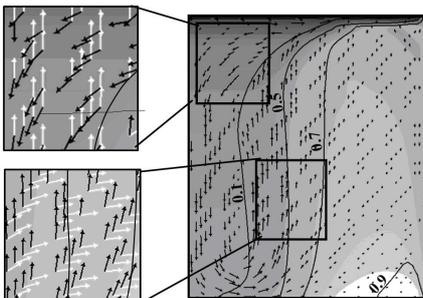
Fig. 4 Analysis of the formation of  $c_{mix}$  at 150 s. Black arrows:  $\bar{u}_\ell$ . White arrows:  $\nabla c_\ell$ .
