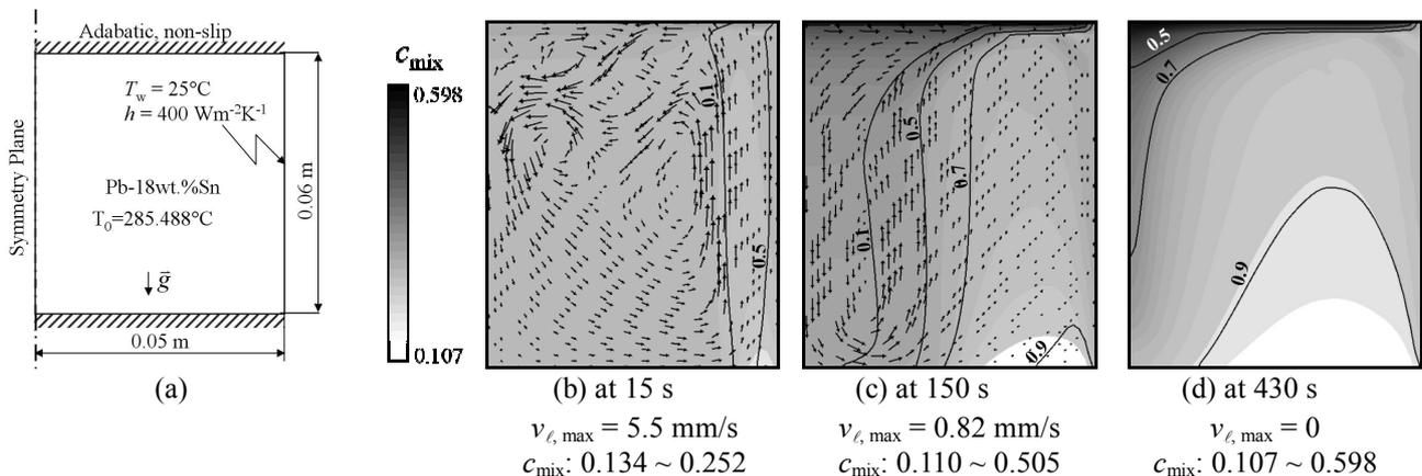
Fig. 1 (a) Configuration of the benchmark problem [1]. (b-d) Solidification sequence at 15 s, 150 s and 430 s. The evolution of macrosegregation  $c_{\text{mix}}$  is shown in gray scale, liquid velocity  $v_l$  in vectors and  $f_c$  in iso-lines.
