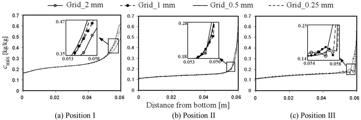
Fig. 3 Comparison of  $c_{mix}$  calculated with a grid size varying from 2 mm to 0.25 mm plotted along lines I to III marked in Fig. 2a.
