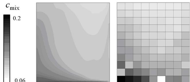
Fig. 5 Simulation of the  $c_{mix}$  in a Sn-10wt.%Bi casting (left) and compared with the experimental result (right) [6].
