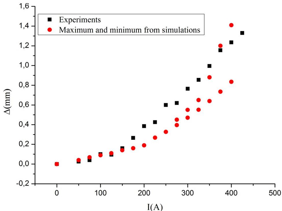
**Figure 4:** Predicted against experimentally observed cavern depths for the case of 4 mm electrode diameter. In the simulations the position of the interface is unstable for  $I > 275$  A.
