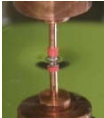
**Figure 2:** Picture of the surface of the liquid metal. A plastic gain of pink colour surrounds the tip of the electrode. A dark area near the electrode appear when the cavern becomes deep and wide enough.
