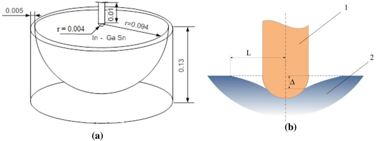
**Figure 1:** (a) dimension of the facility. (b) Scheme of surface deformation  $\Delta$  – depth of cavern, L – width of cavern, 1 –electrode, 2 – liquid metal In-Ga-Sn.
