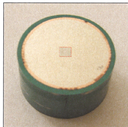
Fig. 4: Embedded St52-sample (sample: grey square in the centre)
