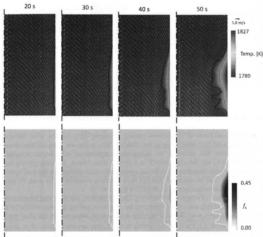
**Figure 3.** Evolution of clogging and its interaction with solidification. The temperature and flow fields are shown on the top row and the solid fraction of steel is indicated on the bottom row. The thick and thin solid lines represent the clog front and liquidus iseline (indicating solidification front), respectively.
