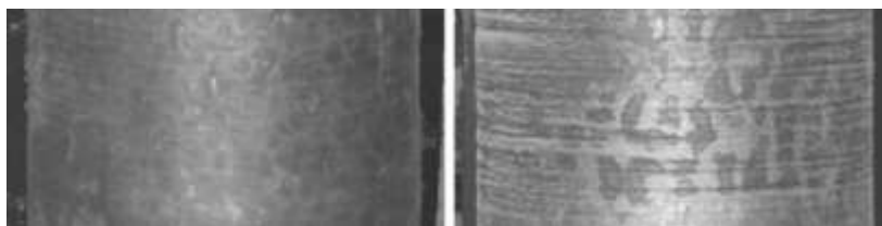
Fig. 6: Example of ingot surface aspect using a) a shallow and b) a deeper immersion
