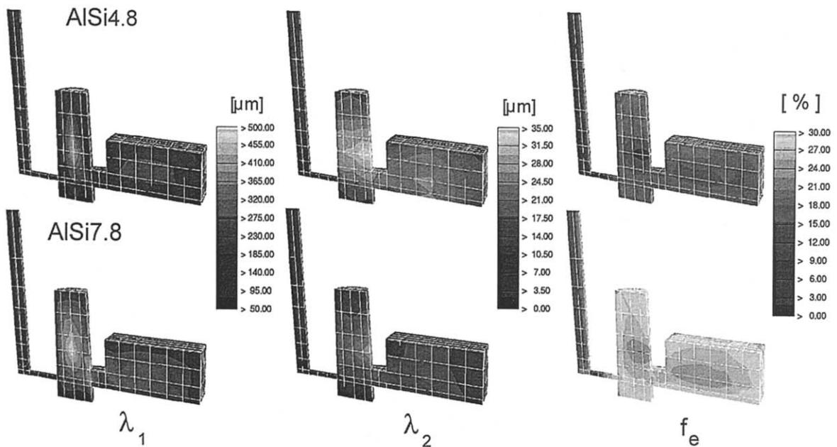
Fig. 5. Primary ( $\lambda_1$ ), secondary ( $\lambda_2$ ) dendrite arm spacing and fraction eutectic ( $f_e$ ) for the alloys Al-4.8 wt.% Si and Al-7.8 wt.% Si under identical initial and cooling conditions. Notice, that in both cases the minimum in  $\lambda_1$  does not correlate with the maximum in  $f_e$ .
