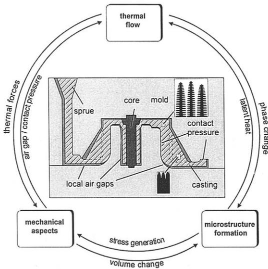
Fig. 1. Various aspects of a coupled modelling of a casting process.
