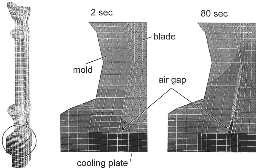
Fig. 3. Development of a local air gap of a complex cast part. The left figure shows a sectional view of an enmeshed turbine blade with cooling plate and ceramic mould. The figure on the right depicts the evolution of a local air gap during directional solidification of the blade. For reasons of clarity the deformations are magnified by 100 times.
