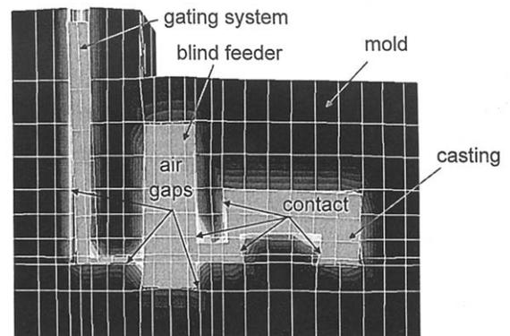
Fig. 4. Example showing the mechanical interaction between casting and mould. Zones with and without air gaps are clearly visible. To illustrate the distortion the displacements have been multiplied by a factor of 150.
