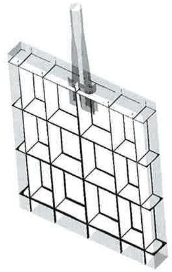
Figure 8. Slice planes through the mould domain showing the solidified shell (black) and the melt pool (white).
