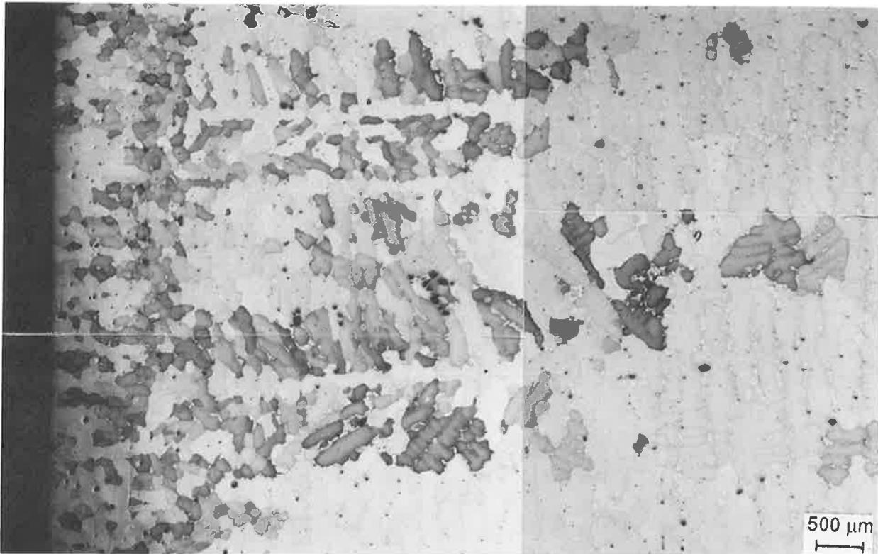
Fig. 4. Enlarged view of the transition region from equiaxed grained into dendritic structure. It can be seen that the origin of the primary dendrite trunks is within the equiaxed zone. Secondary arms develop further towards the end of the transition region.
