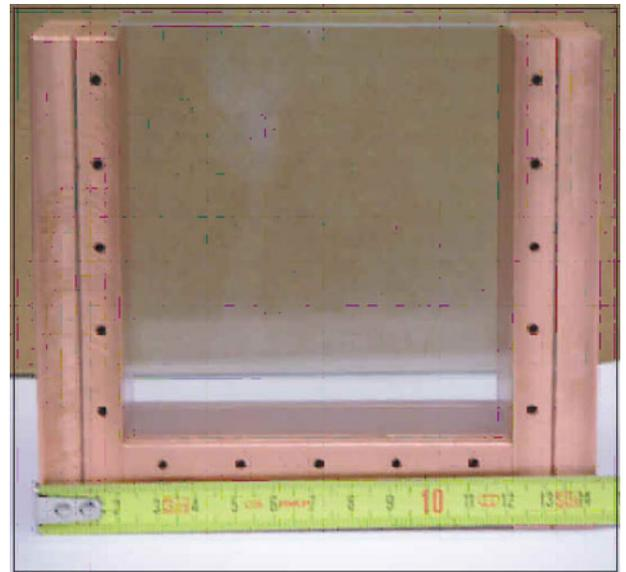
Fig. 1—Rectangular cavity used for the controlled solidification experiments. The inner dimensions are 10 × 10 × 1  $\text{cm}^3$ .
