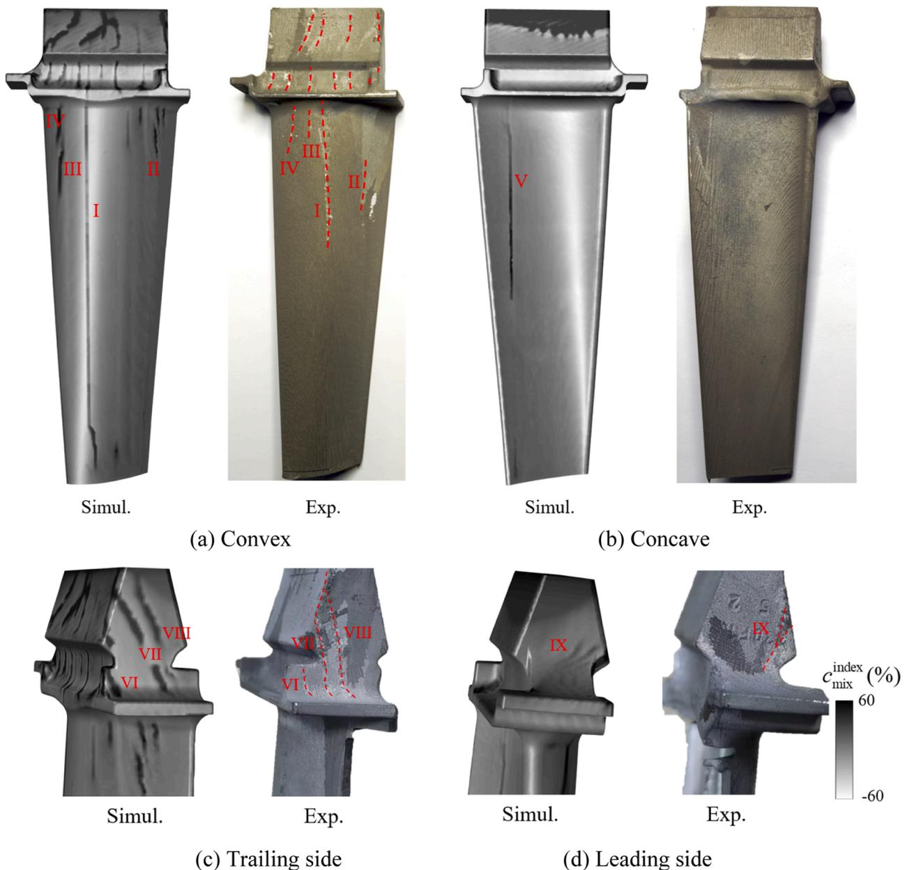
Fig. 9. Simulation–experiment comparison of the freckles in the as-solidified TB. Freckles appearing at different positions are numbered I–IX.
